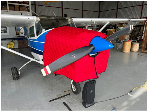
Insulated Hangar Blanket on Cessna 182
