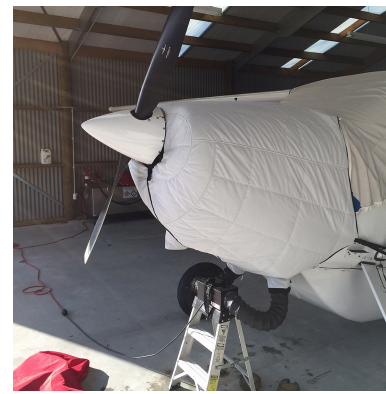
Cessna 180 Insulated Engine Cover with Heater Hose Detail
