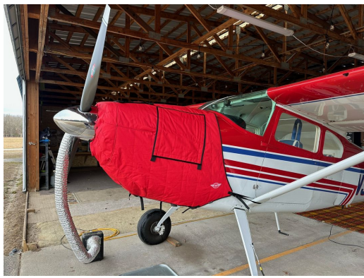
Cessna 180 Insulated Engine Cover, Does Not Cover Bottom
