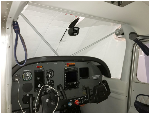
Cessna 180 Skywagon Windshield Heatshield, (W/ Compass)
