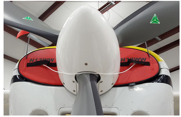
Cessna 180/185 Skywagon Engine Inlet Plugs
