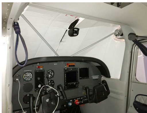
Cessna 180 Skywagon Windshield Heatshield, (W/ Compass)
