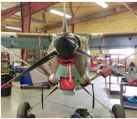
Siai Marchetti 1019 Engine Plugs, Prop Tie-Exhaust Covers
